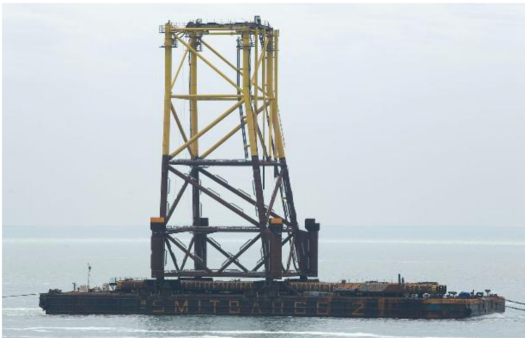
The RT MAGIC departed with the SMITBARGE 2 from Flushing Sloehaven , the barge was loaded with the Chevron A/12 jacket with a weight of 1100 ton. Photo : www.maritimephoto.com
