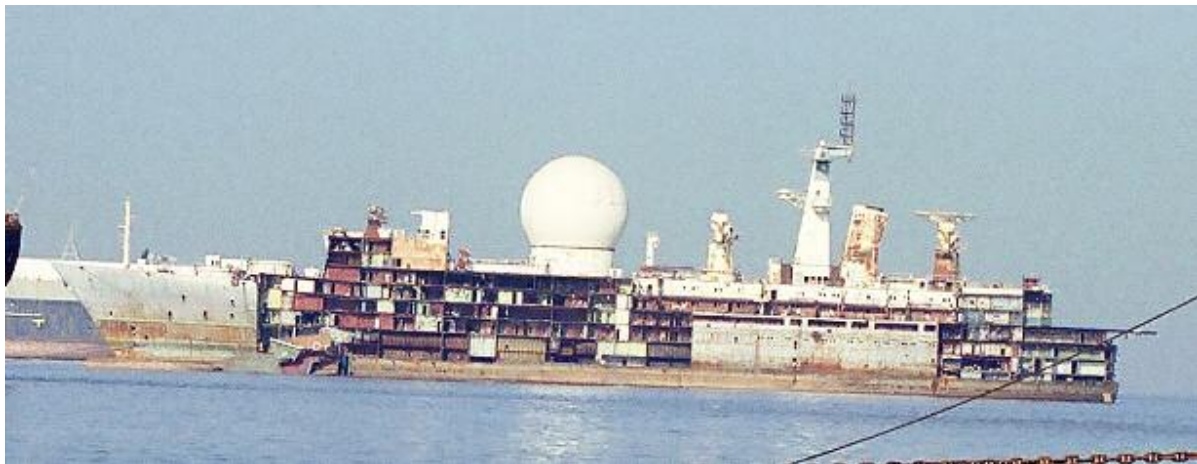
The USSR build in the eighties 2 Space-event ships of the MARSHAL NEDELIN class , the first one was called MARSHAL NEDELIN (1984) and the second was called MARSHAL KRYLOV (1989), the vessel were having a displacement of 25,300 tons full load and dimensions of 211.2 x 27.7 x 8.3 meters, powered by 2 diesels with a total output of 16.000 bhp the vessels were able to make a speed of 22 knots , Crew: 403 persons
