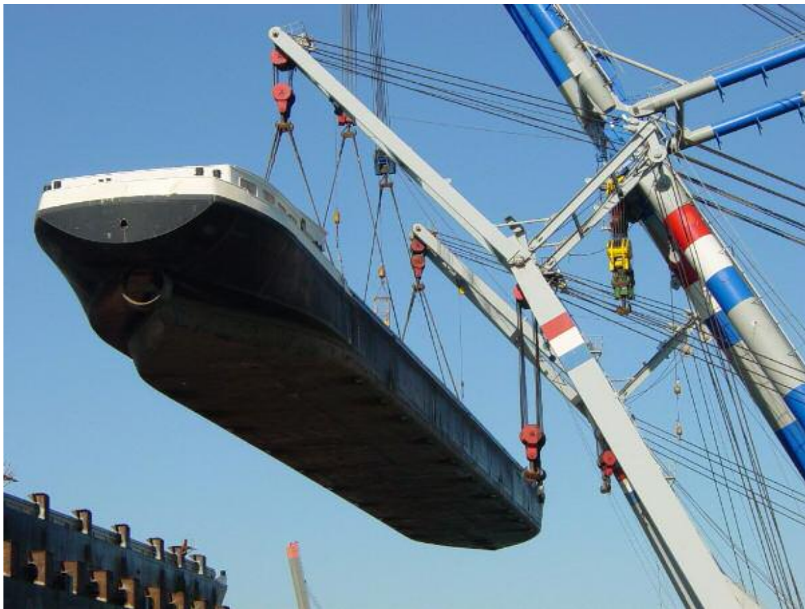
In the port of Rotterdam the highest casco was offloaded from the Sainty no 4 by 3 Bonn & Mees sheerlegs Photo : Aad van Zon ©
