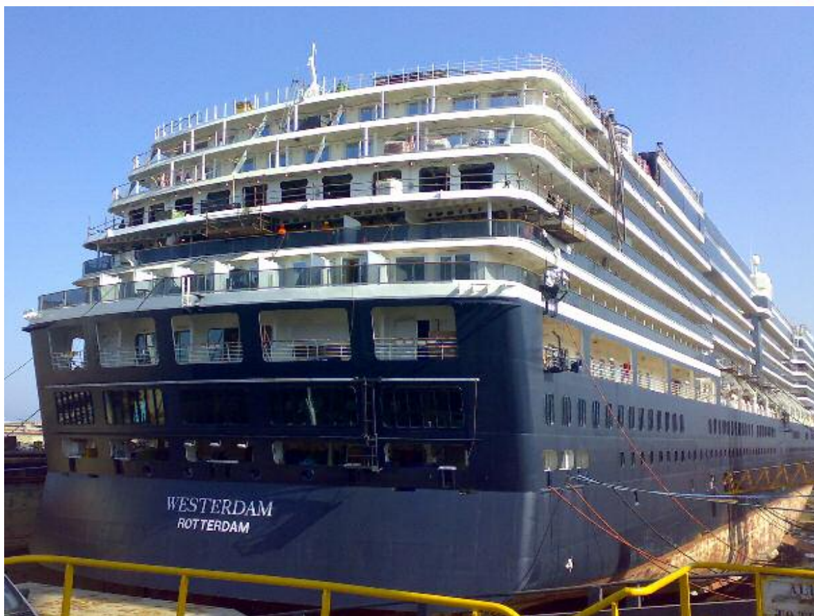
Above seen the new aft section added to ms Westerdam currently undergoing her " Signature of excellence " in dry dock at the Fincantieri yard, Palermo.
