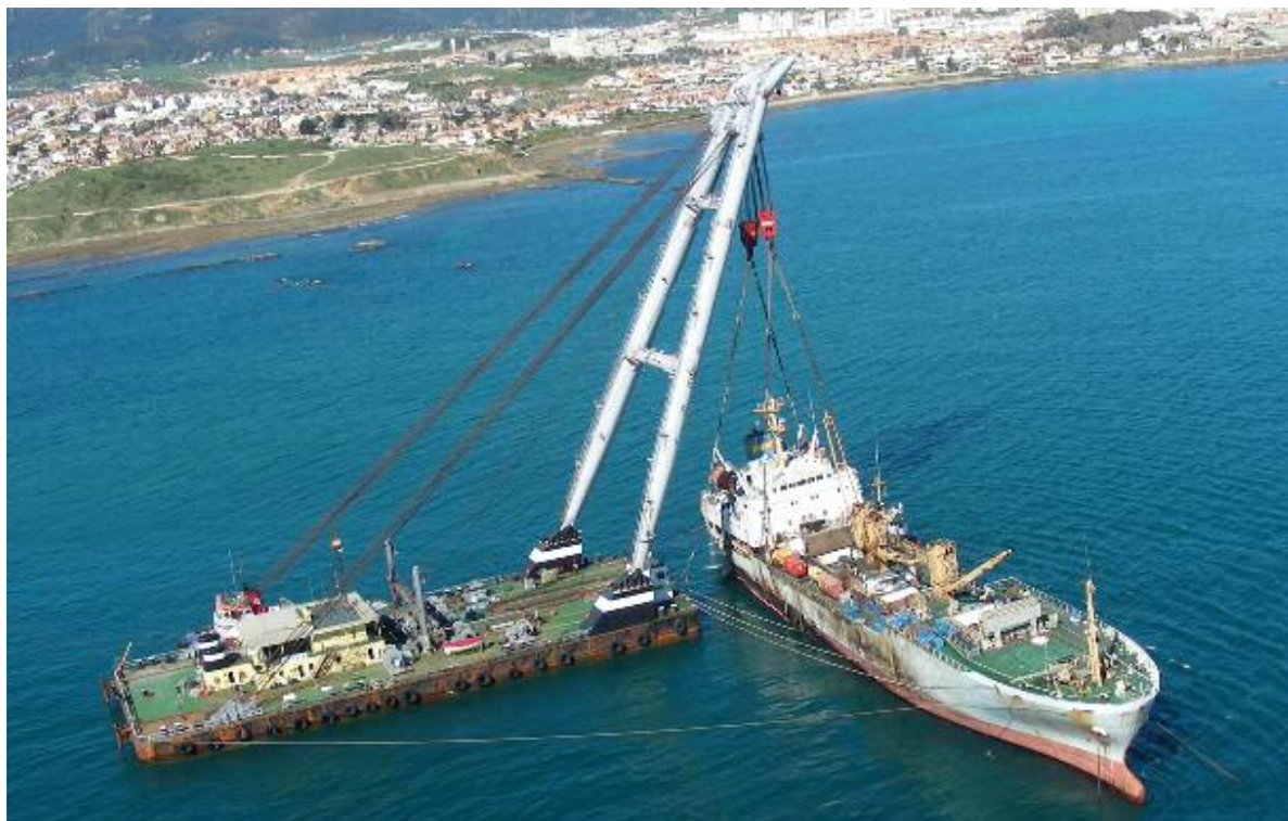
NERI's sheerleg ITALIA seen working on the grounded SIERRA NAVA in Algeciras Photo : via Corrado Neri ©
