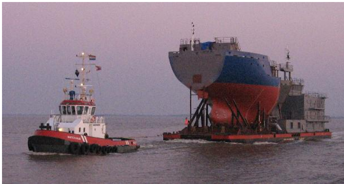
The tug Watergeus seen with the Wagenborg barge 1 , loaded with 800 tons superstructure transported from Volharding location Hoogezand to Volharding location Harlingen.
