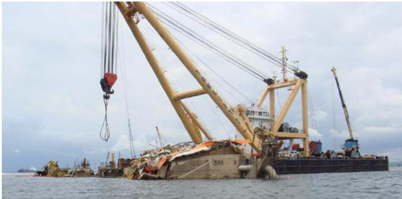
The TAKLIFT 7 seen in action with the refloating of the Boskalis dredger NAUTILUS in Congo, after righting up the dredger was refloated and delivered in the port.
