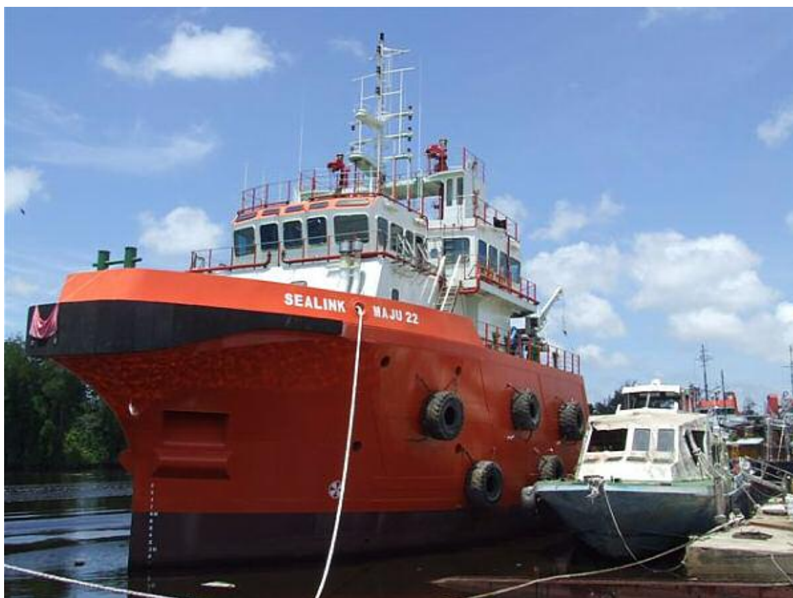
The 4600 hp SEALINK MAJU 22 (60 ton Bollard Pull) seen getting ready for her first dancing steps, the AHTS measures 48 mtr in length and is having a beam of 13.2 mtr.
