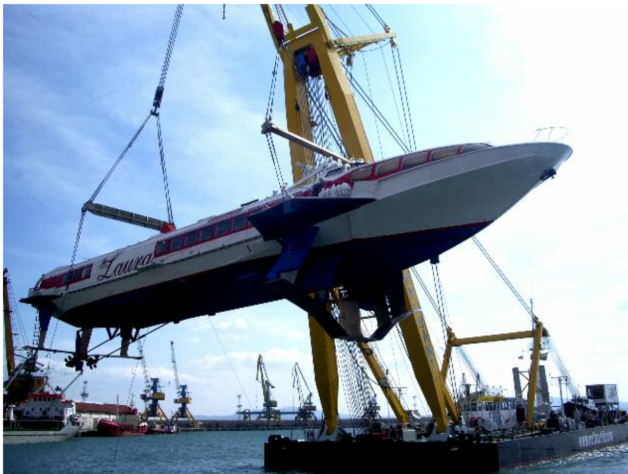
The Hydrofoil LAURA seen here getting discharged from a cargo vessel into her element By the Multraship's sheerlegs CORMORANT Photo : Pepijn Nuijten - Multraship ©
