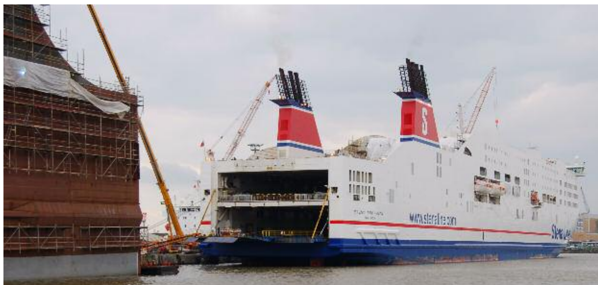
The STENA BRITANNICA seen in Bremerhaven nearing completion, whilst the new mid-section for the STENA HOLLANDICA is ready to be installed.
