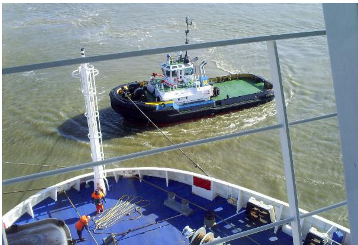
The SMIT MERSEY seen assisting the STENA HOLLANDICA , note the connection made to the SMIT Bracket at the forecastle of the STENA HOLLANDICA Photo : Marianne van der Elst ©
