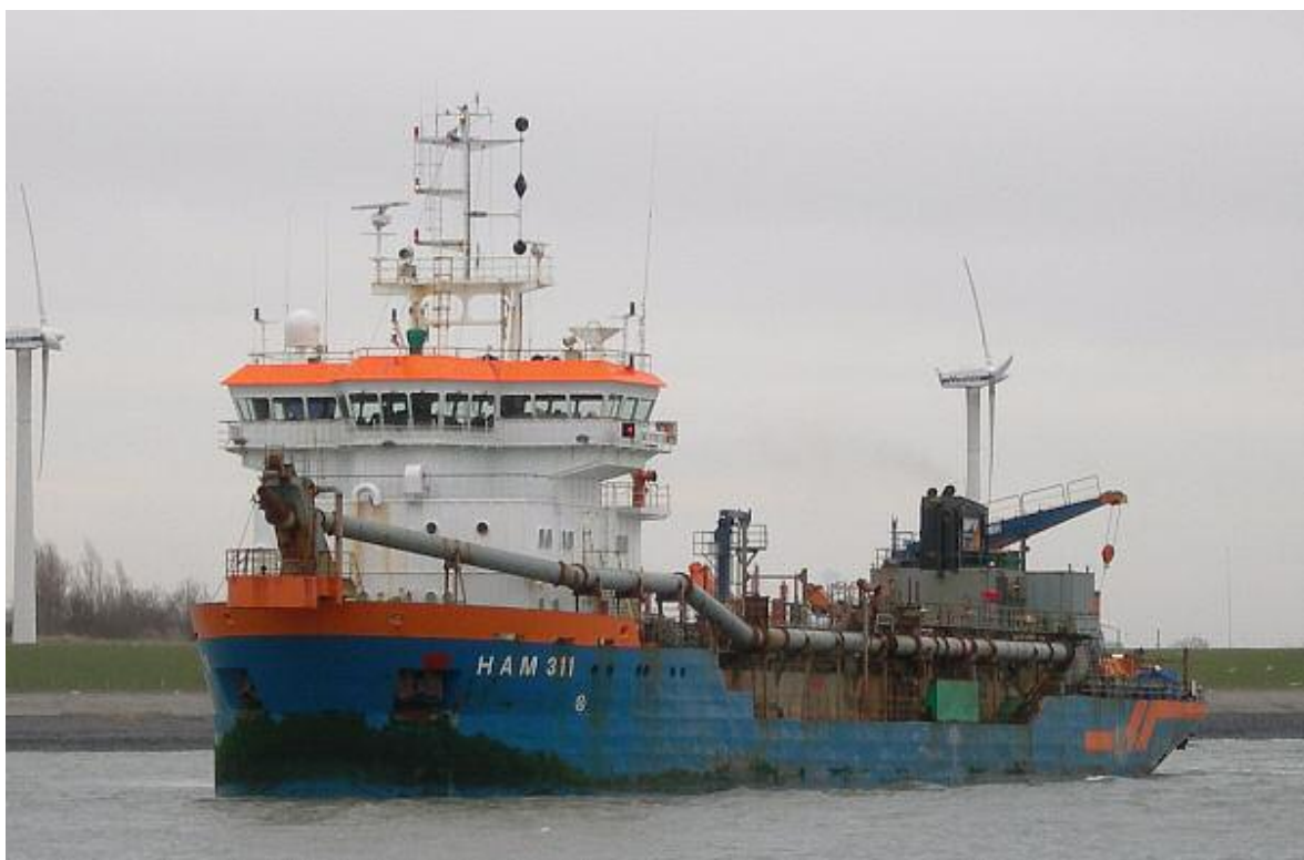
The Trailing suction dredger HAM 311 seen operating in the port of Flushing Photo : Jack Geluk ©
