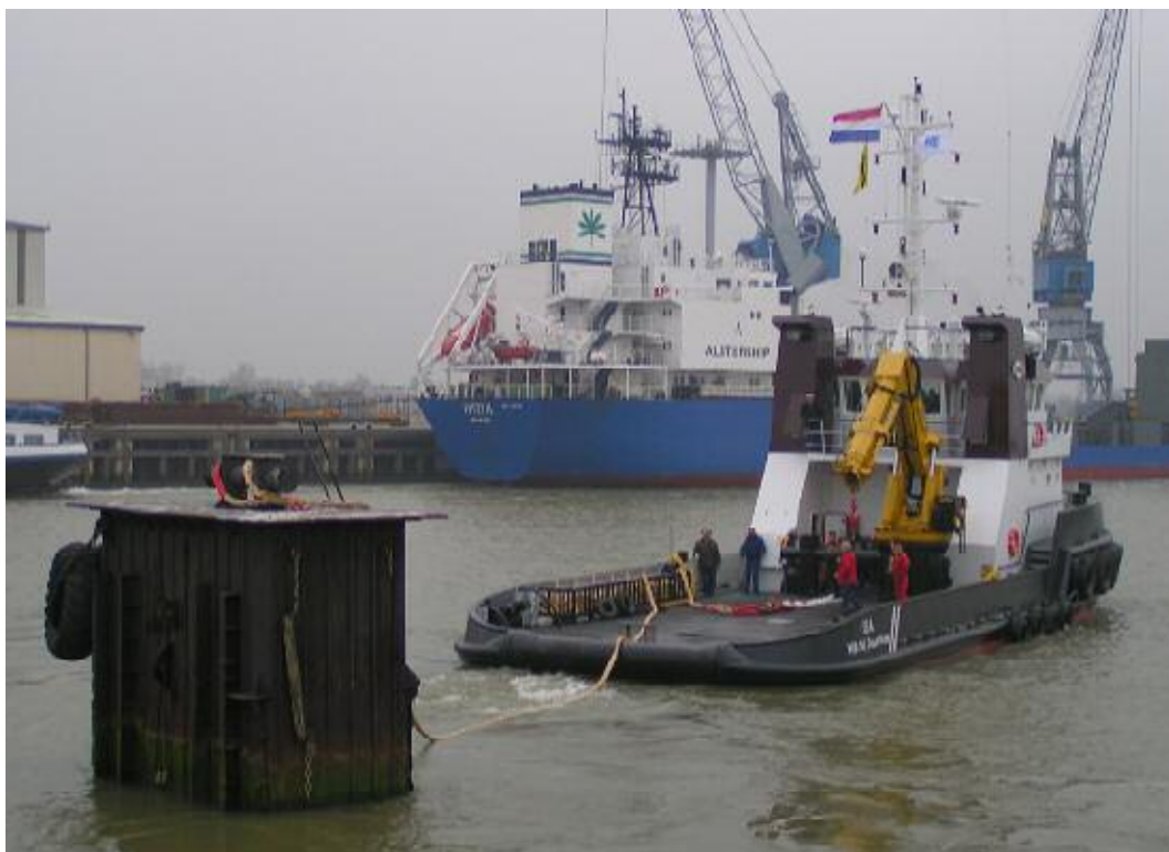
The tug ISA seen during bollard pull tests – Photo : Will Kik ©
