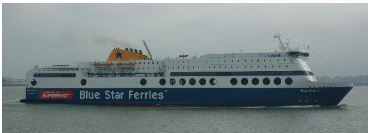
The BLUE STAR 1 is replacing the SUPERFAST X at the route Zeebrugge-Rosyth, the BLUE STAR 1 is built in The Netherlands during 2000 and is just a little larger then the SUPERFAST X , measures a length of 176 mtr and a beam of 25.7 mtr, her service speed is 28 knots, and is able to carry 840 passengers, 640 cars + 100 trucks.
