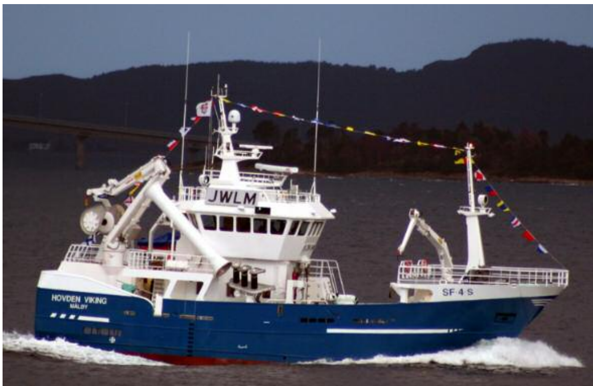
The newbuilding " Hovden Viking " seen arriving at Aalesund for christening. This 90 feet purse seiner, NC 90, is designed by Naval Consult and built by Larsnes Mek. Verksted as hull no 44.
