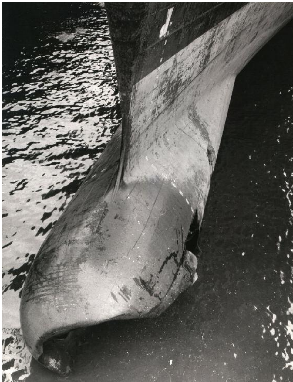
The Atlantic Crown , after a contact at full speed with a growler at the North Atlantic, in drydock at Wilton Fijenoord. March 1975.
