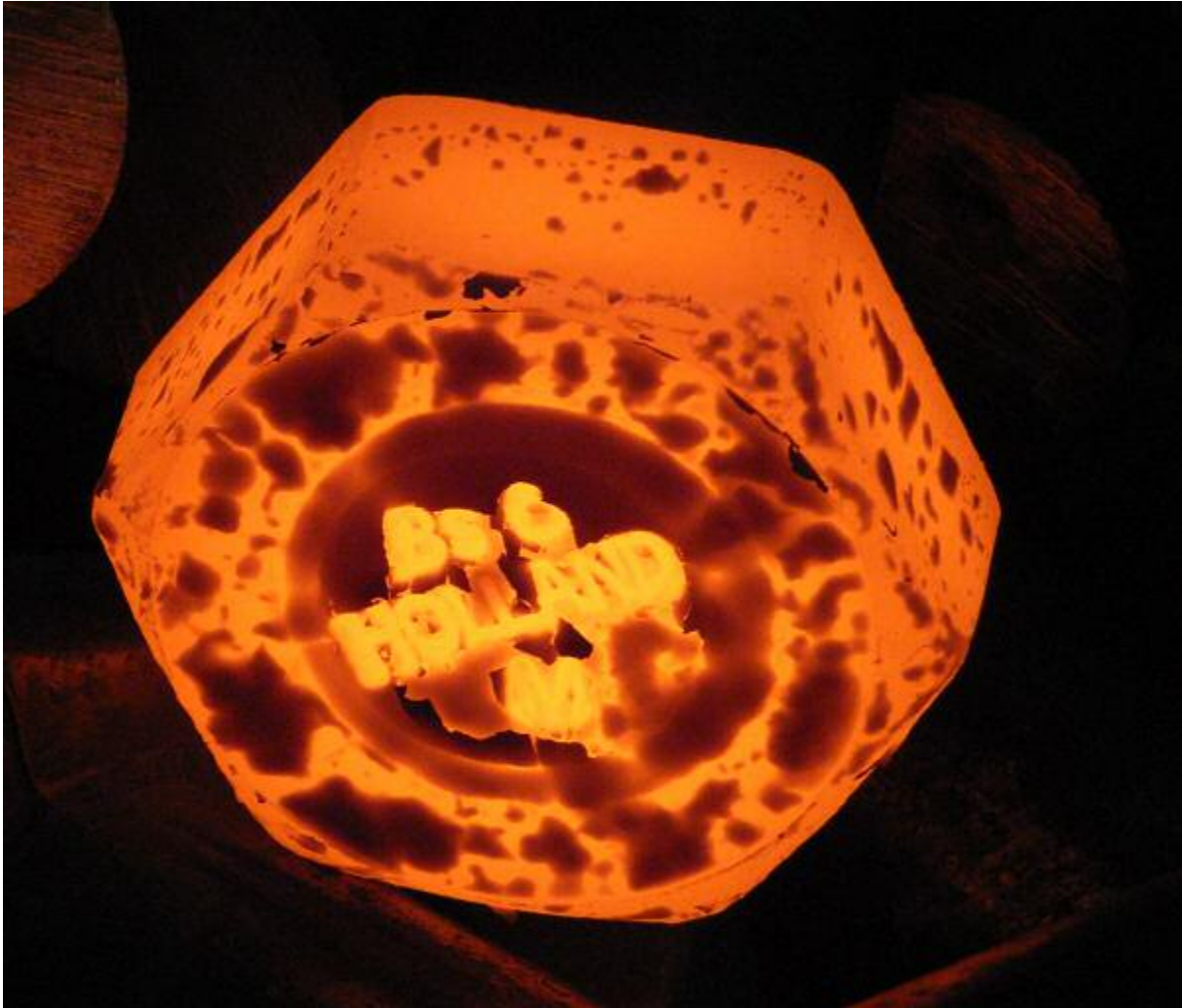
A shackle pin for an original GREEN PIN shackle heated up / under construction at the Van Beest shackle factory in Sliedrecht (The Netherlands)
