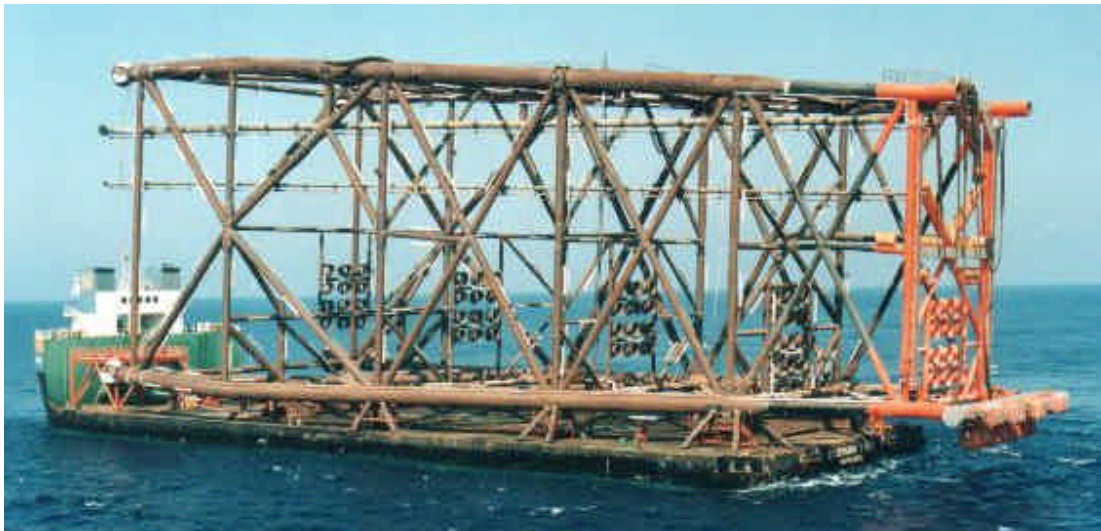
The SMIT ANAMBAS loaded with the TEMSAH 4 jacket – photo : Hans van der Ster ©
