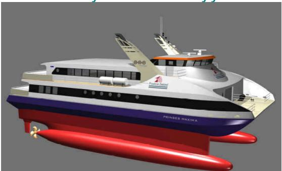
**Prinses Maxima**, the first of two new Small Waterplane Area Twin Hull (SWATH) ferries being built by Damen shipyards in the Netherlands for the Province of Zeeland is due to be delivered by the end of this year, followed by the second ship in the series, the **Prins Willem Alexander**, which is due to be delivered early next year. Both vessels are due to enter service by March of 2004.
