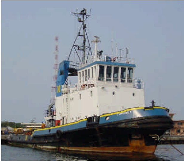
The tug COURBET was build during 1983 and has a power of 3100 hp, she measures 40.2 mtr x 10.5 mtr with a GRT of 494 ton.
