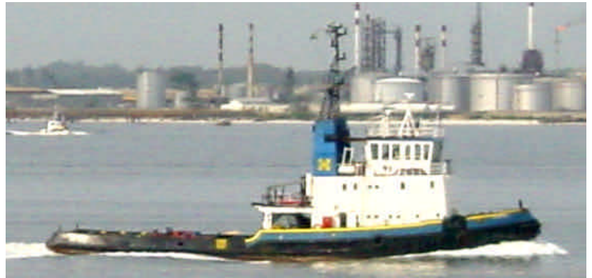
The tug COURBET was build during 1983 and has a power of 3100 hp, she measures 40.2 mtr x 10.5 mtr with a GRT of 494 ton.
