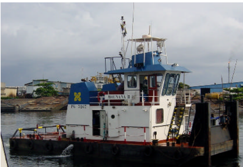
Right : The 1350 HP Makokou was build during 1975 and measures 22.1 x 6.8 mtr with a GRT of 94 tons.
