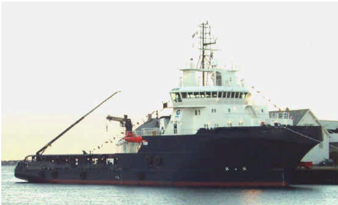
Top : The 16320 BHP HIGHLAND ENDURANCE with a Bollard pull of 180 tons
