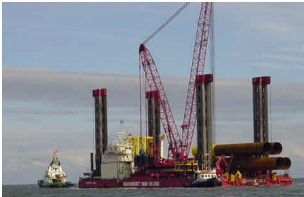
The Jack up platform JUMPING JACK enroute the construction site for the new to build windmill park offshore Great Yarmouth
