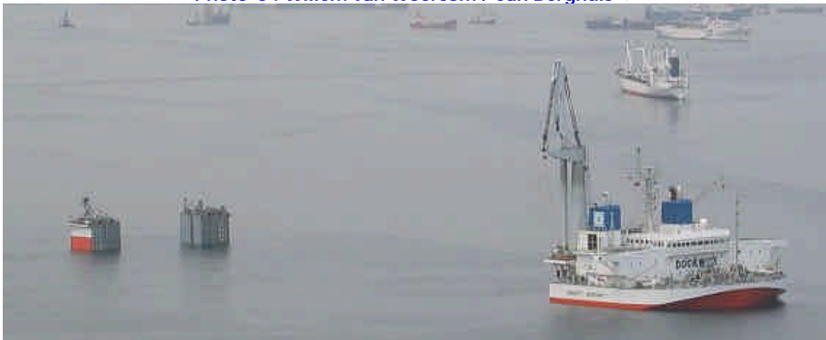
The KIZOMBA-A platform was floated-off the Mighty Servant 1 offshore Luanda
