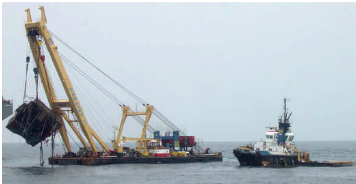
The sheerlegs TAKLIFT 1 assisted by the tug VIKINGBANK seen here lifting a part of the sunken rig ROWAN HOUSTON in the Gulf of Mexico – photo : Jaap Striegel ©
