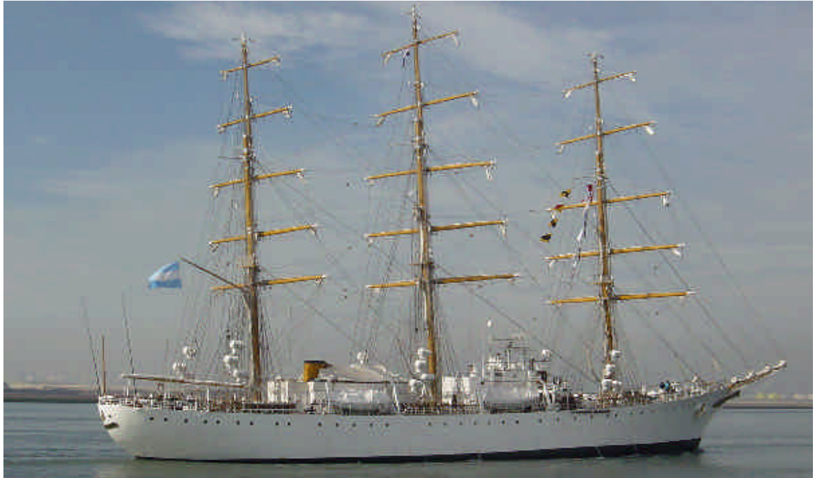
The Argentine sail trainer LIBERTAD departed from Rotterdam – photo : Piet Sinke © The foremast is 48.66 m high, mainmast 50 m, and mizzen 43.17 m.
