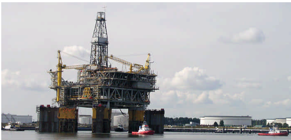
Top : The KIZOMBA-A platform have left the building location and is seen here at the 7 th Petroleum harbour during stability tests, the platform was hold in position by the tugs ZP Montelena , ZP Chandon , Smit Rhone, Smit Clyde and Smit Humber .
