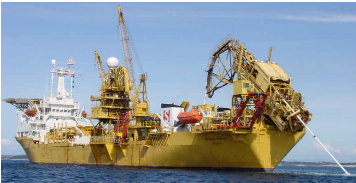
Top : The SEAWAY FALCON laying a 10" pipe at the Rogass job.
