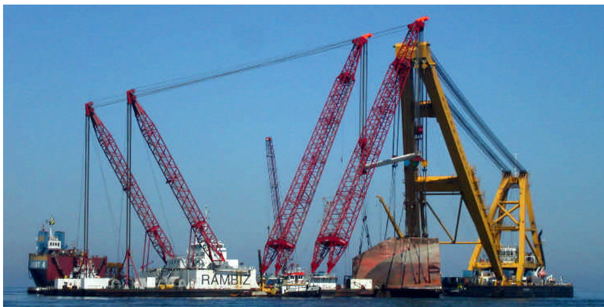
The first part ( section 9 ) of the TRICOLOR being lifted by the ASIAN HERCULES II and RAMBIZ onboard the GIANT 4 - photo's : Danny Spaans ©
