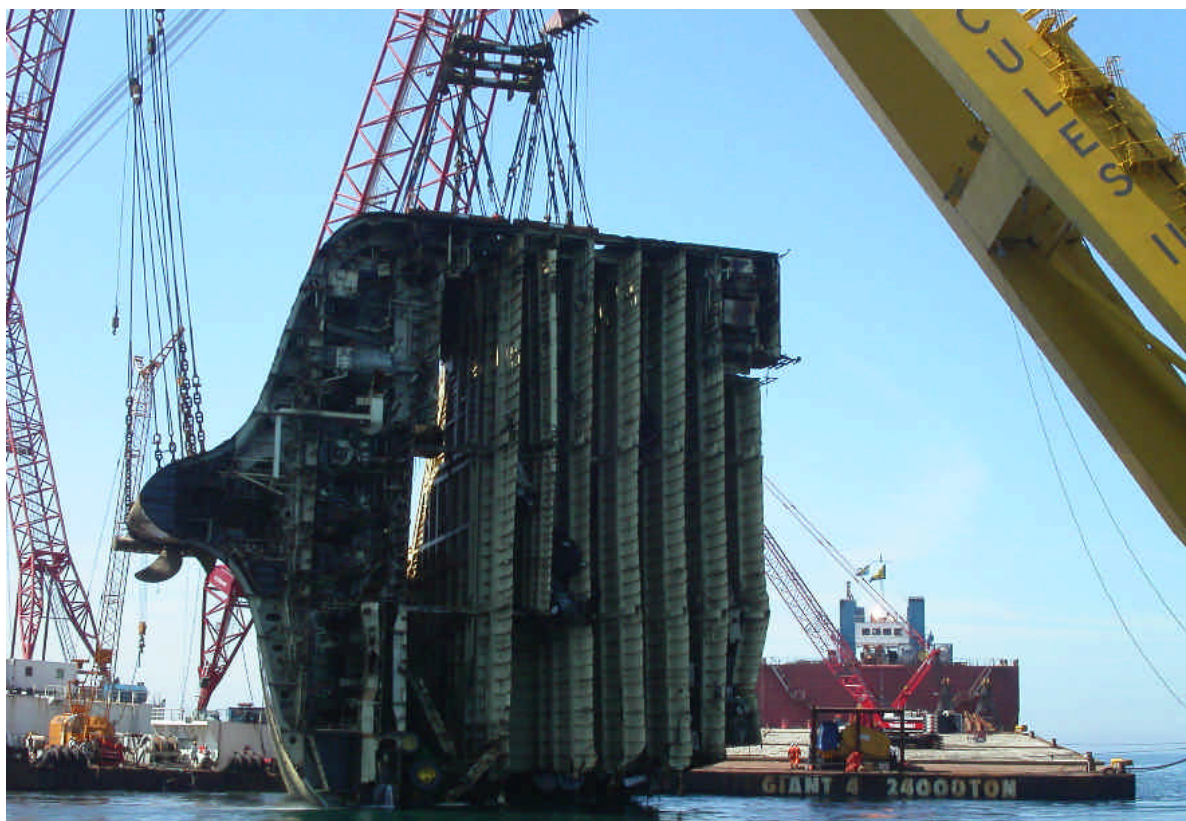
The first part ( section 9 ) of the TRICOLOR being lifted by the ASIAN HERCULES II and RAMBIZ onboard the GIANT 4 - photo's : Danny Spaans ©
