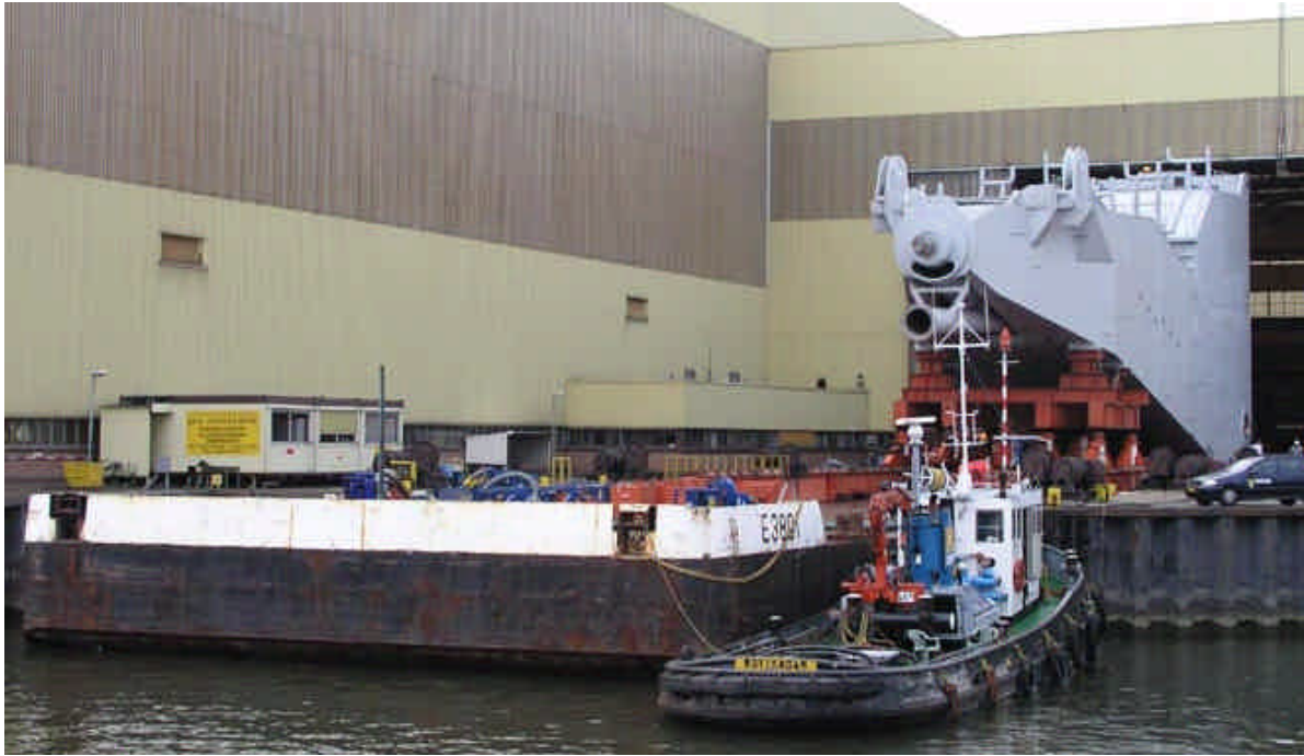
The ladder is skidded outward of the building location Photo's : Hans de Jong Maritime Pictures ©
