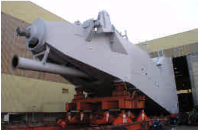
The ladder is skidded outward of the building location Photo's : Hans de Jong Maritime Pictures ©
