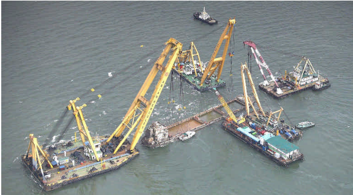
Smit Salvage mobilised units and salvage crew to the sunken TIRTA MAS during the third week of April 2003. Four sheerlegs were deployed to raise the casualty, Asian Hercules , Smit Typhoon , Asian Helping Hand III and a Semco crane . Tirta Mas was officially redelivered to its owner's (on recovery site) on 18 June 2003. photo : Smit Singapore ©
