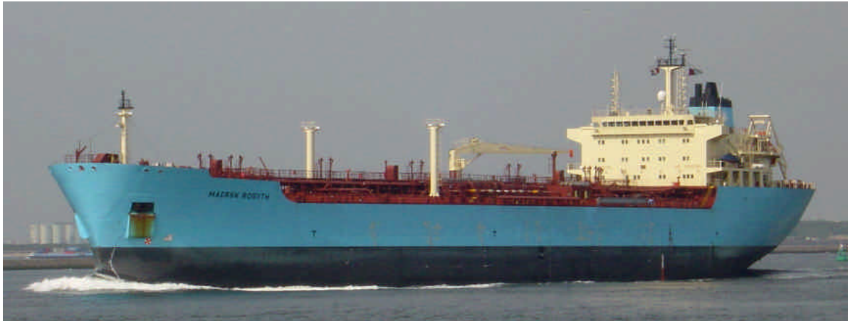
The MAERSK ROSYTH seen here arriving in Rotterdam – Photo : Piet Sinke © A.P.Moller Copenhagen/GBR 2003 Guangzhou GT 22181 dwt 35000 Loa 171.2m Bm 27.4m (JvdK)
