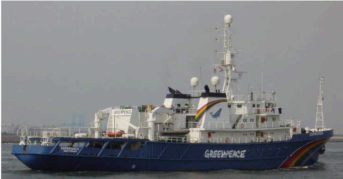
The ESPERANZA Greenpeace Marine Division Amsterdam build during 1984 by Polnocma in Gdansk GT 2076 dwt 425 Loa 72.3m Bm 14.4m 4320 kW ex Vikhr-4 -98, Echo Fighter-01, Eco Fighter-01, Esperanza-02, Echo Fighter-02 departed from Rotterdam 07-06-2003
