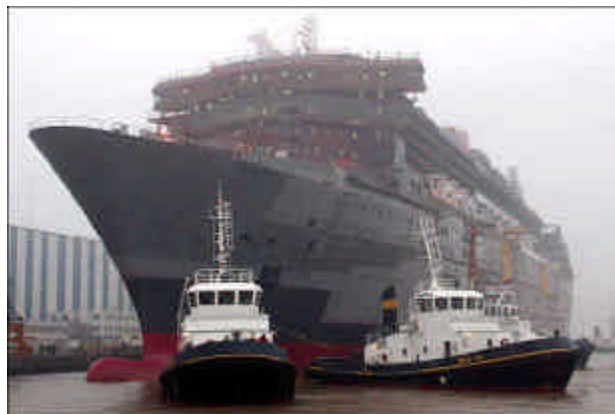
The new QUEEN MARY 2 under construction — photos : via Stefan Roest
