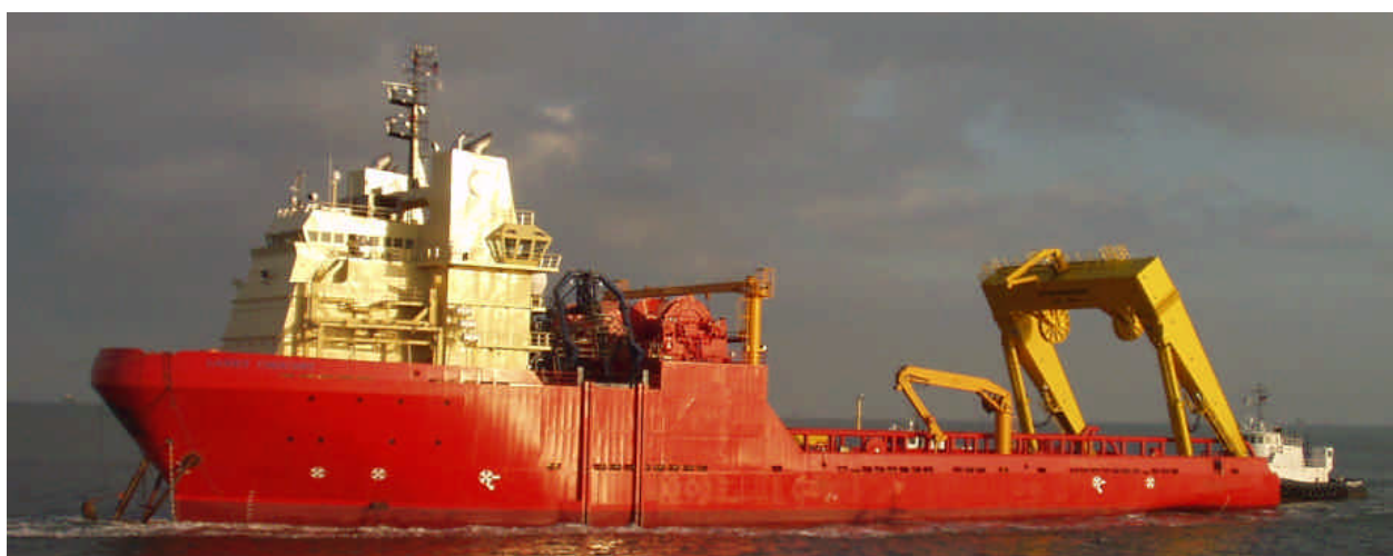
The brandnew LANEY CHQUEST equipped with an A-Frame rated 350 Ton SWL Photo's : Capt Wim van der Kort / Banckert ©
