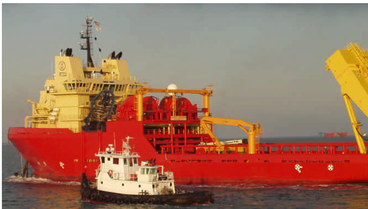
The brandnew LANEY CHQUEST equipped with an A-Frame rated 350 Ton SWL Photo's : Capt Wim van der Kort / Banckert ©
