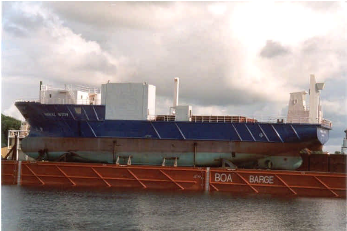
The hull of the MIKAL WITH loaded on a Boa Barge Photo : Olav Moen ©
