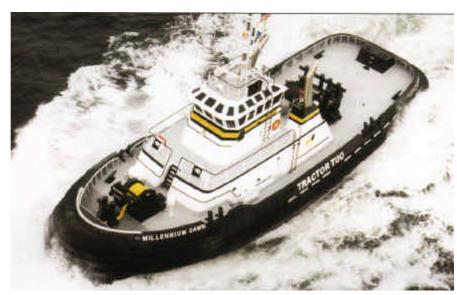
32 x 11.2 x 5.03 (depth ) mtr , 2 Caterpillar 3516B providing 4400 HP which are driving Z-drive units
