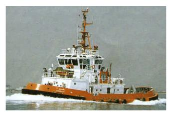
As mentioned before, the three other tugs, **Damman 4**, **Jeddah 31** and **Jubail 28**. are virtually identical except that they have the 6M628 versions of the same engine series, each developing 1270kw at 1.000 revs driving 28G11/I65 Voith propulsors, to give a bollard pull of 35 tonnes, and a unclassified fire-fighting system, again supplied by Counterfire, consisting of Kumera-Norgear driven pumps of 850 m/hr and 600m/hr in a similar arrangement to that of the more powerfull sisters
