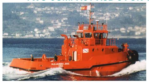
Alejandro Jose and Paula S, a pair of 20m ASDs, are the first tugs to be built by Factoria Naval de Marin in Spain Delivery of the second vessel has just taken place, five months after delivery of her sister, to the Vigobased operator Remolcanosa. Although the tugs are designed for harbour operations with a
