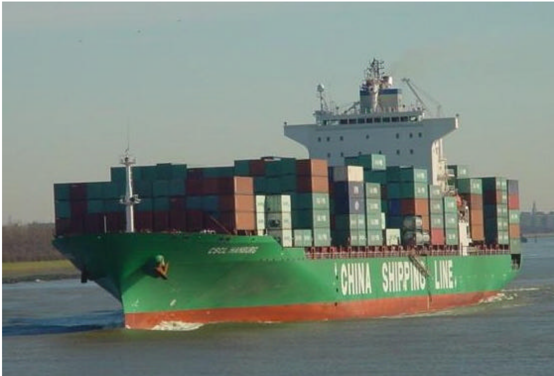
CSCL HAMBURG (9224300) Ofer Brothers Haifa/Cyprus 2001 Samsung Kojie Isl GT 39941 dwt 39600 TEU 4050 Loa 259.8m Bm 32.2m departing from Rotterdam ( Photo/Tekst Jan van der Klooster )
