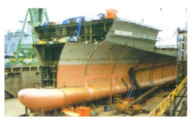
The hull, which has a characteristic delta shape, provides both a large load bearing capacity (up to 16000t) and a stable work platform. This delta-shaped hull form is more fuel efficient at speeds of about 15 knots than similar specification conventional vessels.
