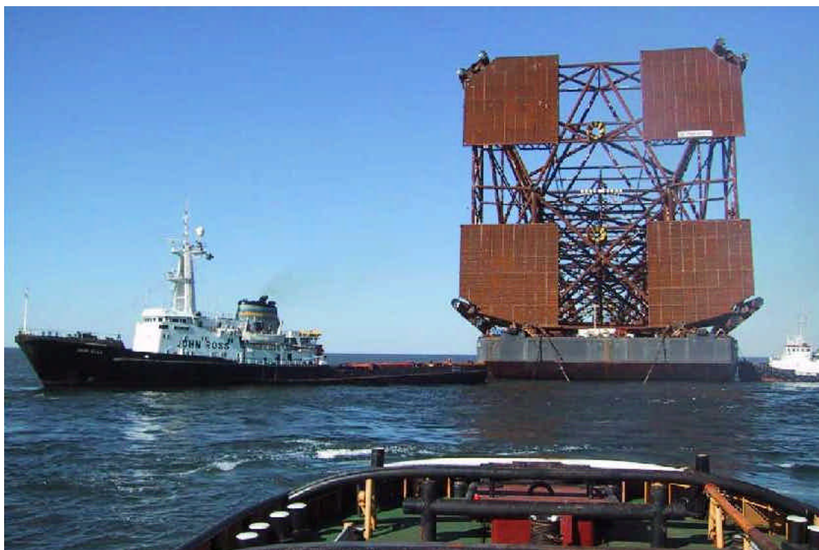
Top : The JOHN ROSS connects her towing gear to the H-851 whilst the SMITWIJS ROTTERDAM is already connected.
