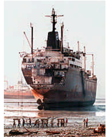
Giants of Alang: Beached merchant vessels dwarf laborers who strip them. Tidal extremes and a gently shelving beach allow shipbreaking without piers or drydocks
