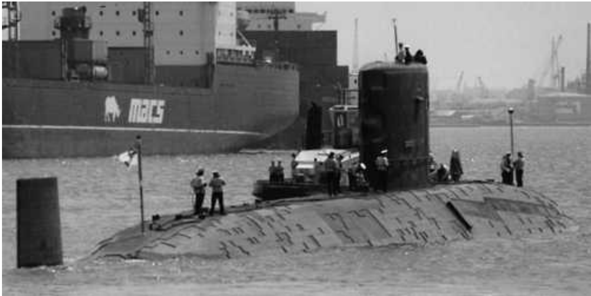
Top : File picture of the TRAFALGAR ( 07-1998 ) with numerous missing anechoic tiles
