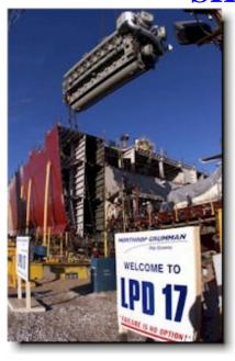
Northrop Grumman Corporation (USA) recently achieved an important milestone in the construction of **San Antonio** when it completed early landing of all four main propulsion engines and three of five power generators on their foundations. In addition, 55 of the 210 units have been erected on San Antonio, the lead ship in the Navy's new LPD 17 Class of amphibious transport dock ships. The ship is scheduled for delivery in November 2004
