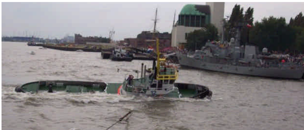
The carroussel tug MULTRATUG 12 during a demonstration under tow of the Fairplay 25
