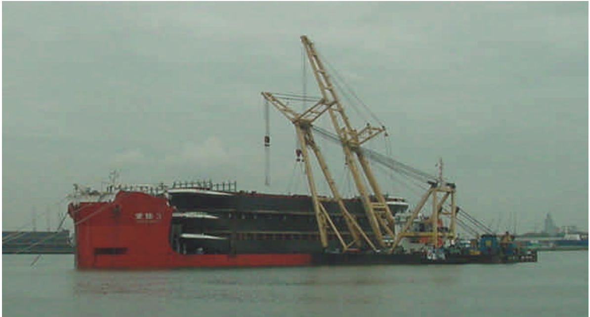
The Taklift 1 and Taklift 7 discharging the in the China build casco s in the Waalhaven in Rotterdam .
