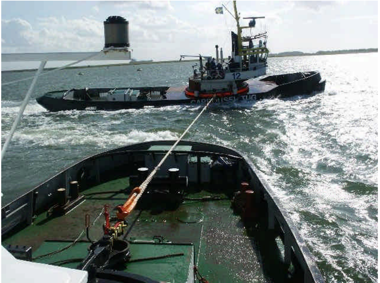
Sailing carrousel - hook over SB-side (85 deg) (approx. 40 tonnes)
