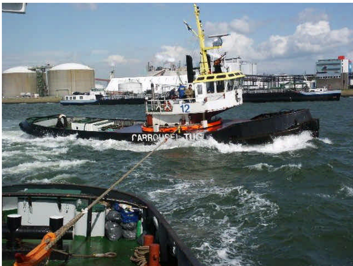
Sailing carrousel - hook over SB-side (110 deg) (approx. 20 tonnes)
