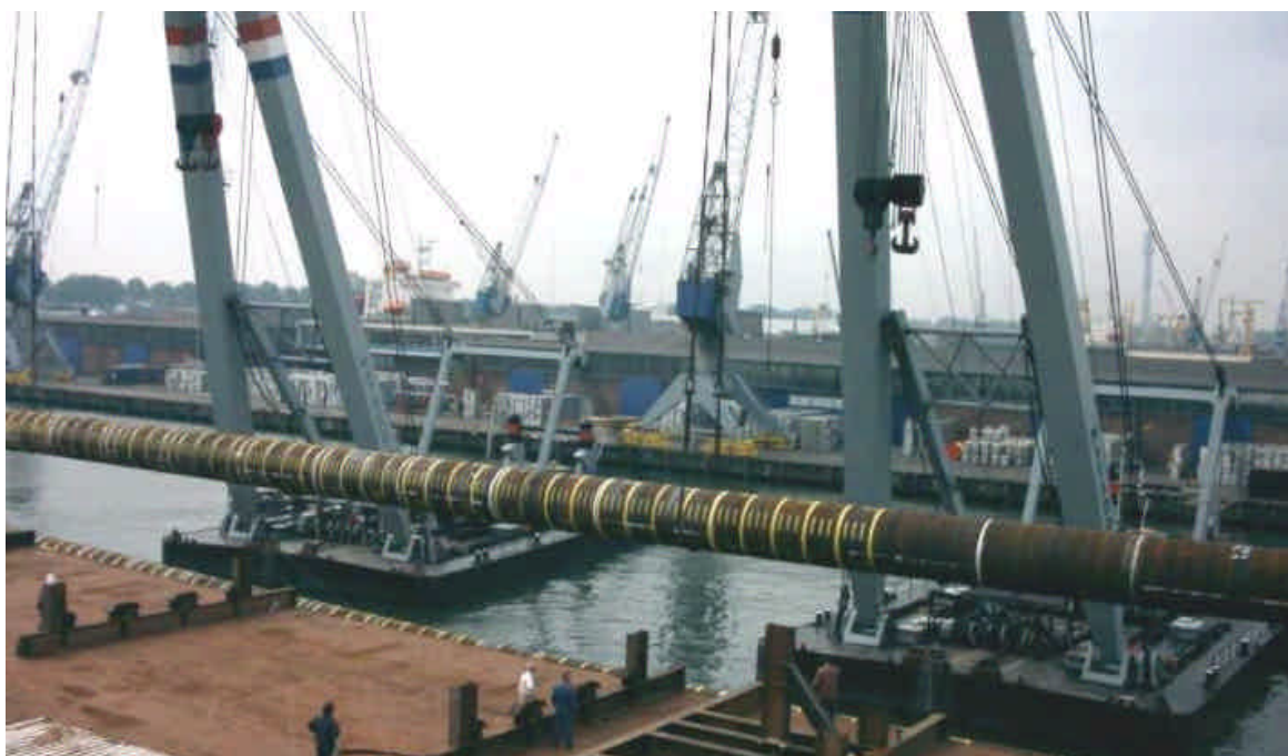
The 2 Matador shearlegs loading a pile onboard the GIANT 2 – Photo : Hans van der Ster ©
