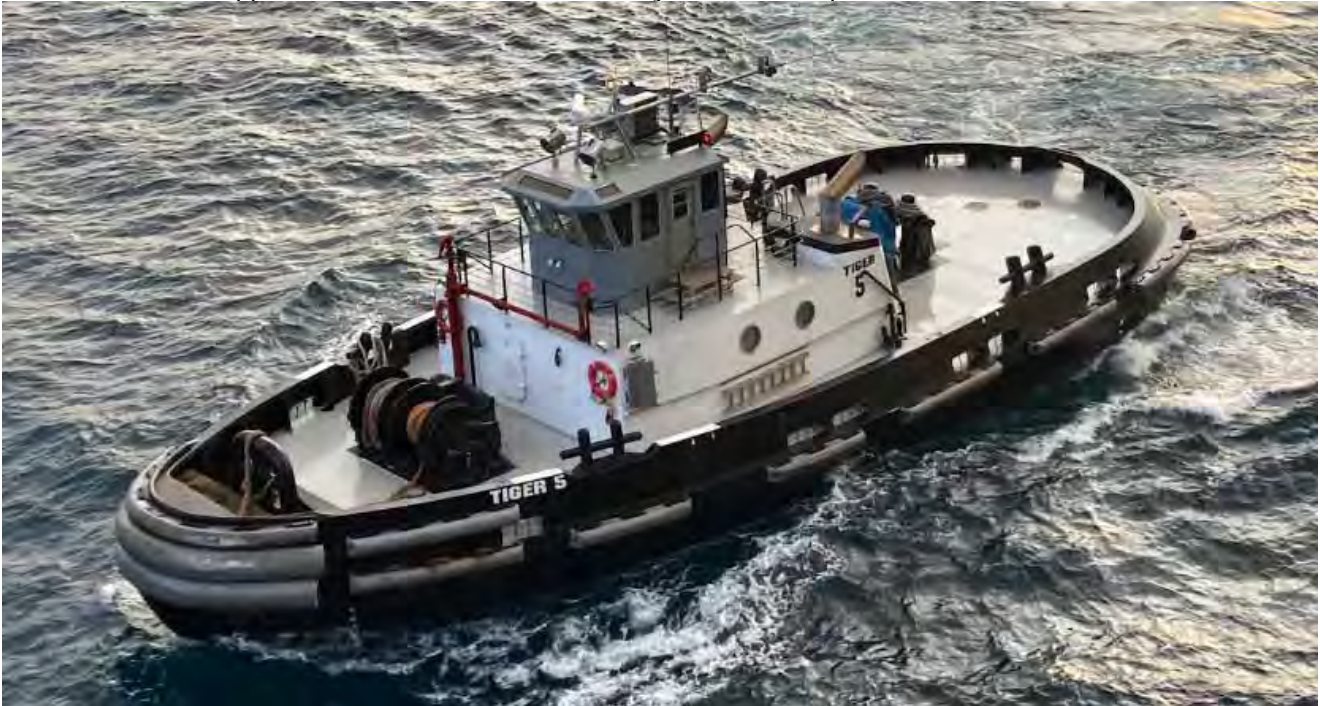
The TIGER 5 an ASD tug of 4400 HP, length 94 ft, beam 34 ft built by Honolulu Marine in 2008 is escorting the KONINGS DAM at Nawiliwili Hawaii. Photo : Harrie Nijenhuis (c)
