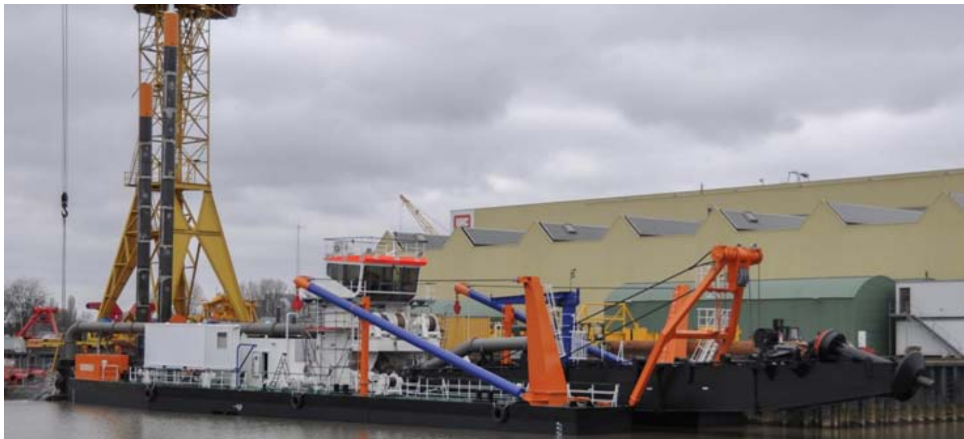
The CSD DE BIESBOSCH seen fitting out at Royal IHC in Sliedrecht, the CSD is under construction for van Oord
