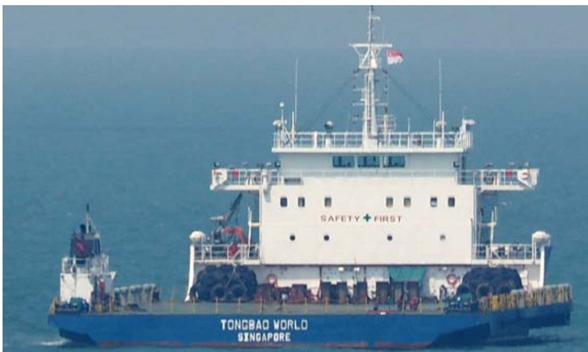
The 2010 built Singapore registered 86 mtr long & 29 mtr width 4289 DWT Heavy load carrier TONGBAO WORLD anchored off Singapore photo : Piet Sinke (c) CLICK on the photo !
