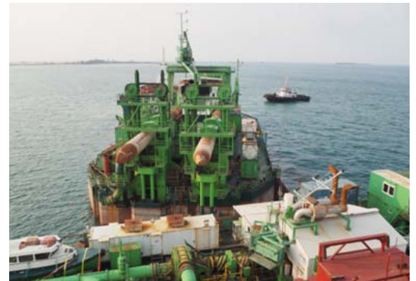
Overnight the FALCON ballasted down to the required draft to be ready at first daylight to discharge the cargo, at sunrise
