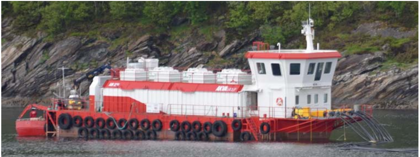
It looks like a pusher tug but the Rodøya is a feeder station for fishfarms operating in Norwegian waters
